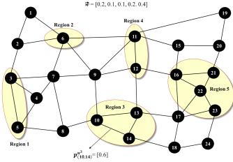
Fig. 5. 24-node test network with |U|=5 a-priori failure regions
