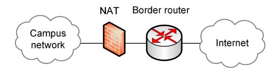
A flow is uniquely identified by the external IP, campus IP, external port<sup>1</sup>, campus port, protocol
