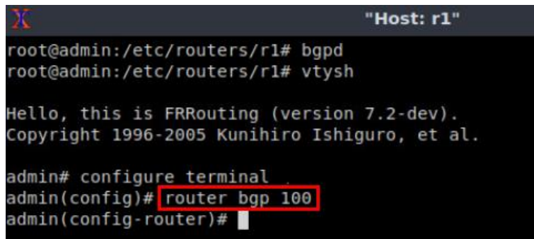
Figure 52. Configuring BGP on router r1.
