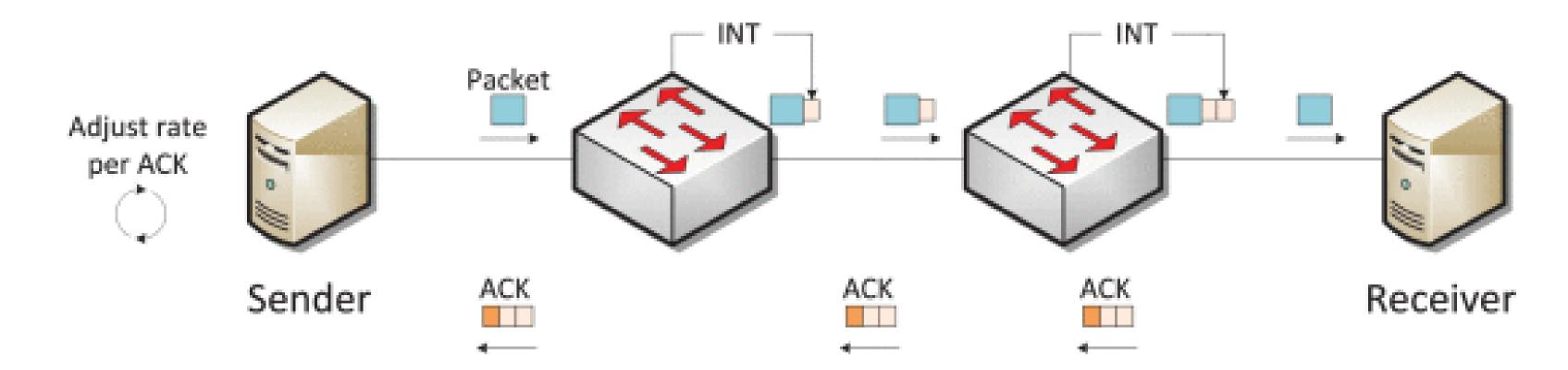
These switches can also be used for load balancing. Typical load balancers work by acting as the webserver, but instead, distributes load amongst real servers. With P4 switches, a server can manage the server pool while the switch forwards the requests. This method increases throughput while decreasing latency.
