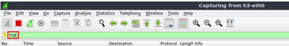
Figure 22. Filtering TCP packets only.
