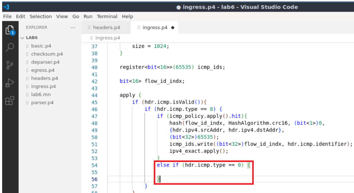
Figure 26. Checking if the ICMP packet is a reply.
