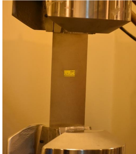
Figure 1 Experimental set up for fatigue crack growth. Cyclic fatigue loading was applied on the specimen by mounting the specimen on MTS machine.
