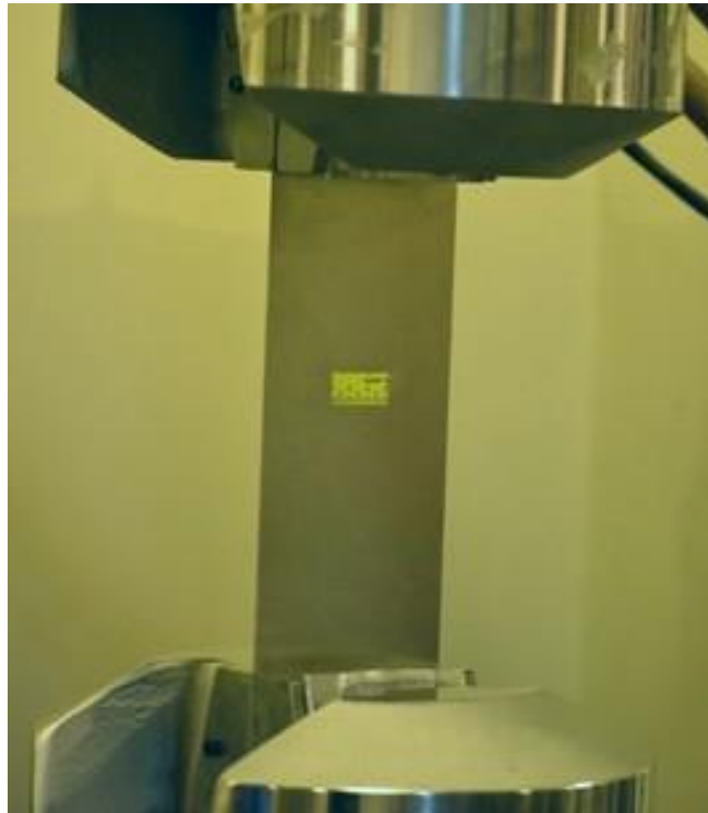
Figure 1 Experimental set up for fatigue crack growth. Cyclic fatigue loading was applied to the specimen by mounting the specimen on the MTS machine.
