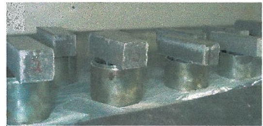
Figure 7 - Primed concrete bricks under the exhaust hood.
