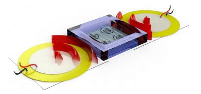
An acoustofluidic particle manipulation platform that uses low frequency flexural waves produced by commercial transducers.
