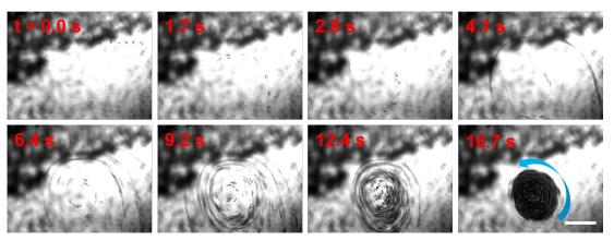
Fig. 3 Frames depicting the particle concentration effect in the acoustic vortex (20  $\mu$ m particles) generated in the flexural-wave-based acoustofluidic device. Using a 5.3 kHz signal applied to both transducers, a rotating mass of particles has formed on the surface of the liquid in the device within 17 seconds. Scale bar: 500  $\mu$ m.
